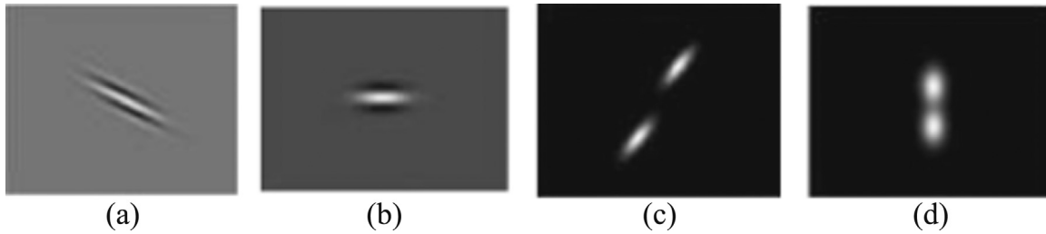
Fig. 3. Gabor filters in spatial domain and frequency domain. (a) spatial response for parameter set P=\{30^\circ, 0.2, 0.5, 1\} . (b) spatial response for parameter set P=\{0^\circ, 0.1, 0.5, 1\} . (c) frequency response for filter in (a). (d) frequency response for filter in (b).
